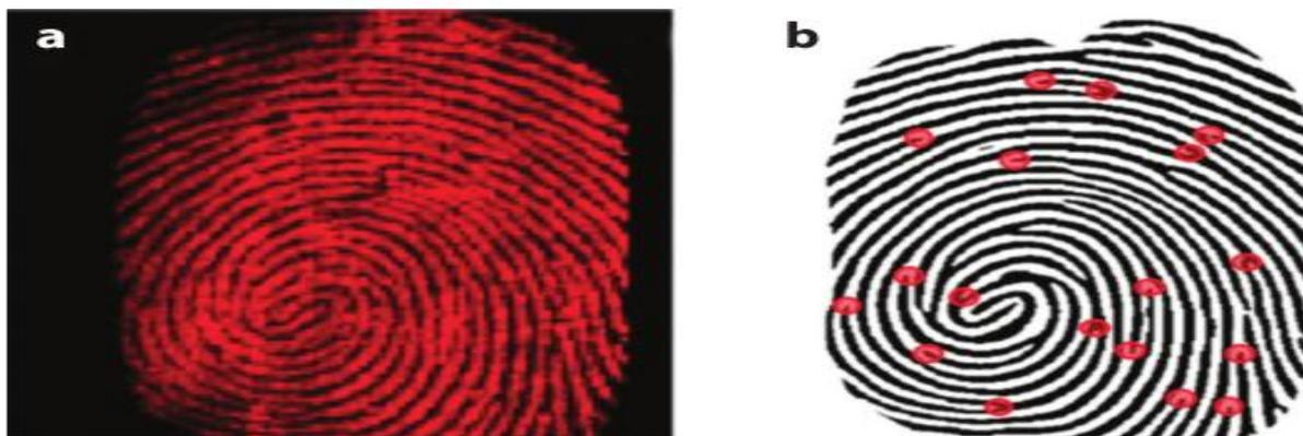
Figure 2: (a) DESI image showing cocaine distribution on a latent fingerprint. (b) Computer-developed fingerprint from DESI image, and the red dots are points of minutiae that are automatically detected. Reprinted with permission from (Ifa et al., 2008).
