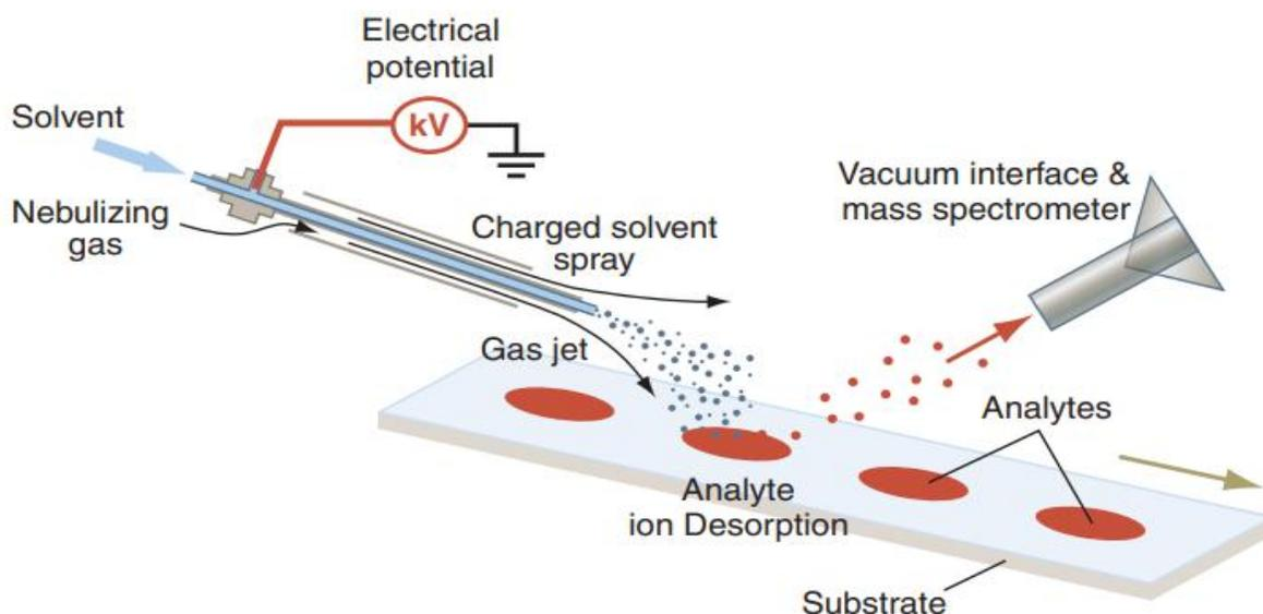
Figure 1: Desorption electrospray ionization for ambient analysis of samples without preparation. Reprinted with permission from (Cooks et al., 2006).
