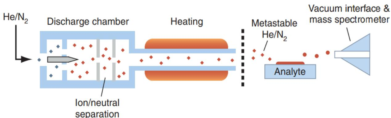
Figure 3: Direct analysis in real time for ambient analysis of samples without preparation. Reprinted with permission from (Cooks et al., 2006).
